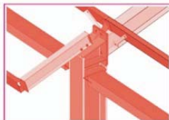
Cornice Connection Point
